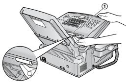
4 Hold the center part of the front cover (①), and pull open the inner cover (②).
